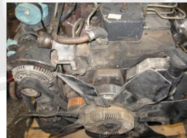
“Old” Style Fan Support and Thermostat Housing
